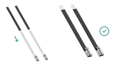
Place the Quick Lock Mount on your frame and feed the two hose clamps through the two gaps in the main body. Then insert the tail end into the opening in the clamp.
